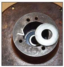
Note the retaining ring that determines the bearing position. The retaining ring is also the stop for the wrought washer againist which the bushing assembly tightens down.
